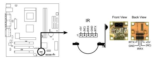
**A7V-M Infrared Module Connector**
